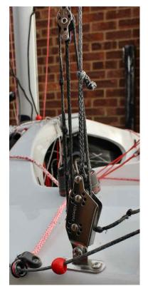
Combined with an adjustable strut, the 'knot system' on the shrouds and a fine tune rig tension led back to the helm has made raking whilst sailing possible. A Ronstan turnbuckle system has made keeping the shroud length equal easy as the knots bed in.
