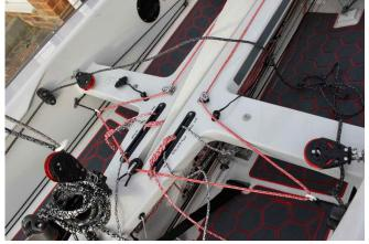
The centreboard control has take ups bringing it to outside of the boat so that again it can be easily found and adjusted by both helm and crew without having to reach inboard or forward.
