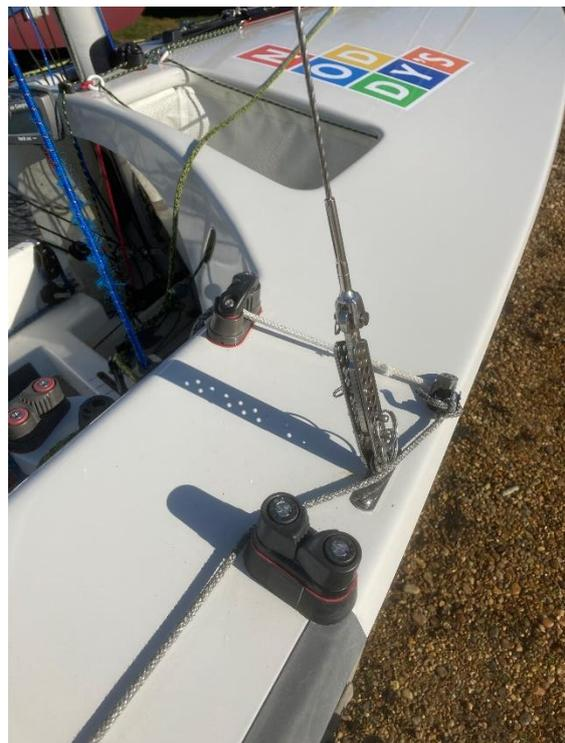
Jib bar system showing simple and calibrated adjustment.
