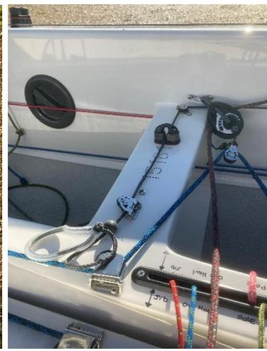
Aft Mainsheet bridal system showing lead to control on thwart.
