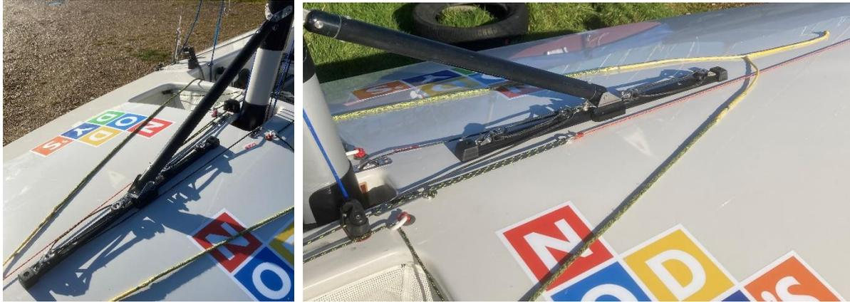
Strut/ Ram system with track on the deck. The jib cunningham line and cleat is also in view.
