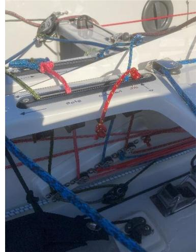
Spinnaker halyard pump cleat show extra cleat to prevent unwanted launching.
