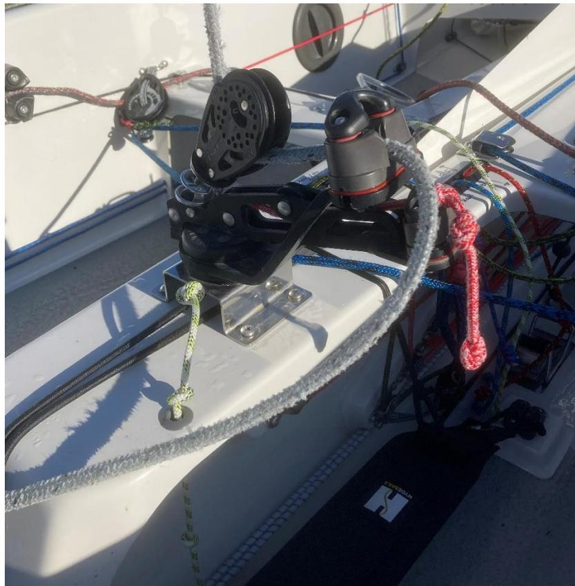
Mainsheet jammer combined with kicker control. Also showing spinnaker bag release line.
