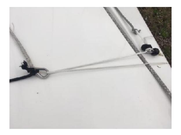
Eye on very short strop through original tails hole. This gives 2:1 at transom with a stopper on the puller line ensuring that the uncleated system provides same geometry as normal tails.
