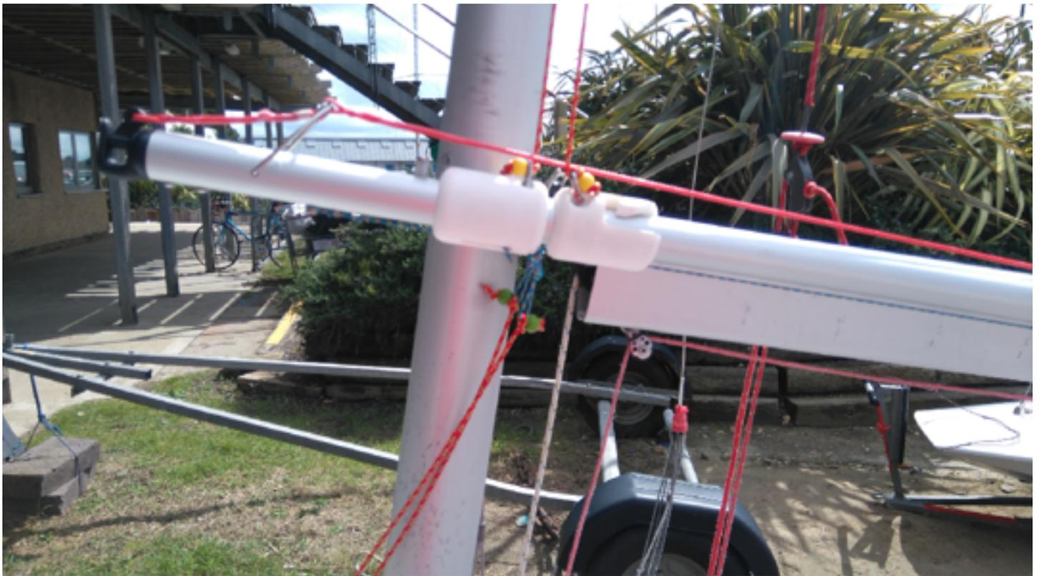
For both the single ended and the Sayce/Rees poles, there are choices with the pole height control. The uphaul(s) can be move so the entry point is higher (~200mm below the jib halyard box?), requiring a sheave fitted here. Alternatively, the uphaul can be fixed to this point and a ring attached to a line entering the mast at the existing sheave point. The uphaul line(s) are passed thru the ring so pulling on the control line puts a kink in the uphaul, effectively shortening it.
