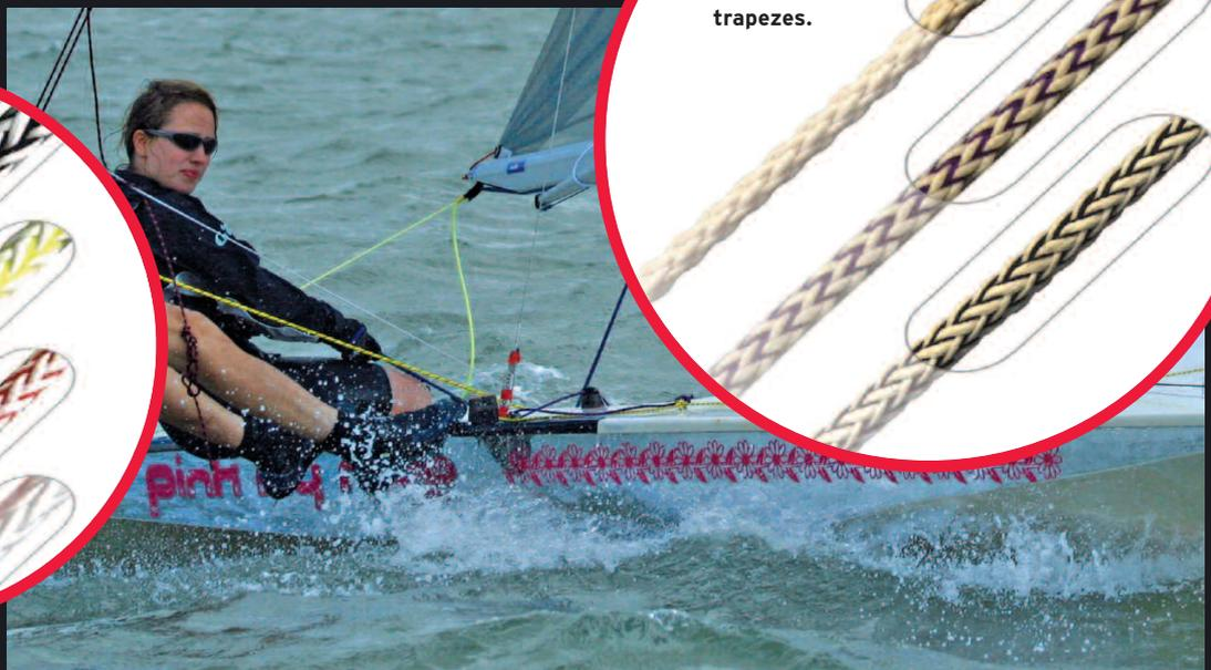
Up high the decision was made to replace the wire trapeze lines with 2.5mm V12, significantly reducing weight with no compromise in terms of strength and elongation. This uncovered 12-strand Vectran line is also easy to splice and is UV-resistant due to Marlow's new Armourcoat high penetration coating, which also provides significantly better wear resistance.
