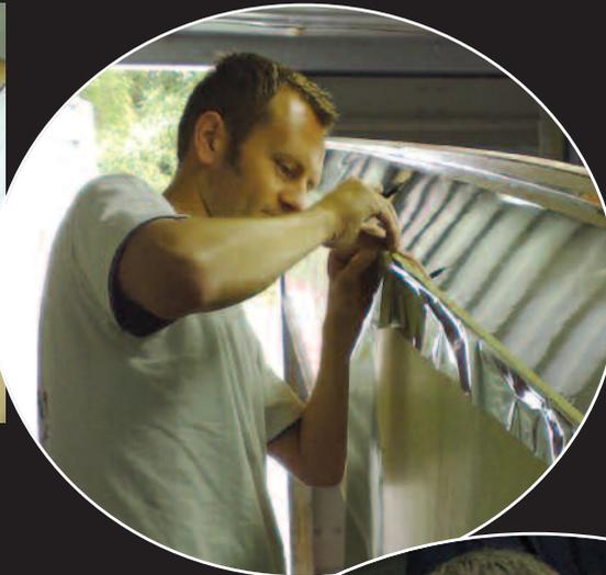
**Left** The chrome was applied by hand. Once stuck down, the excess was trimmed off.
