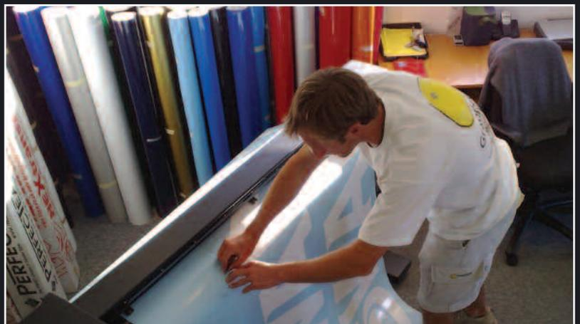
Below The computer is linked to a laser cutter, which cuts the design out of the chosen colour material.
