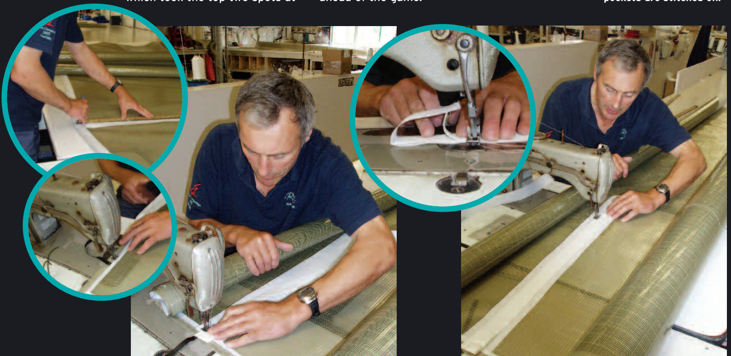
Below Alan Bax shows us how the batten pockets are stitched on.
