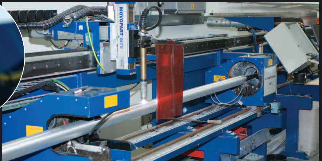
Above and right Step one: the CNC plasma cutter is used to cut the mast taper.
