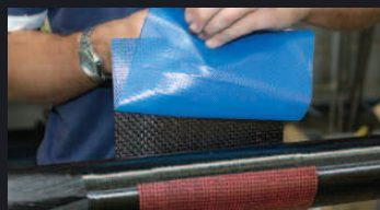
Left The masts are externally reinforced.
