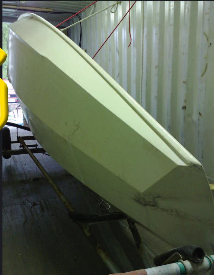
**Right** Gunwale damage needed to be fixed with epoxy and fillers.
