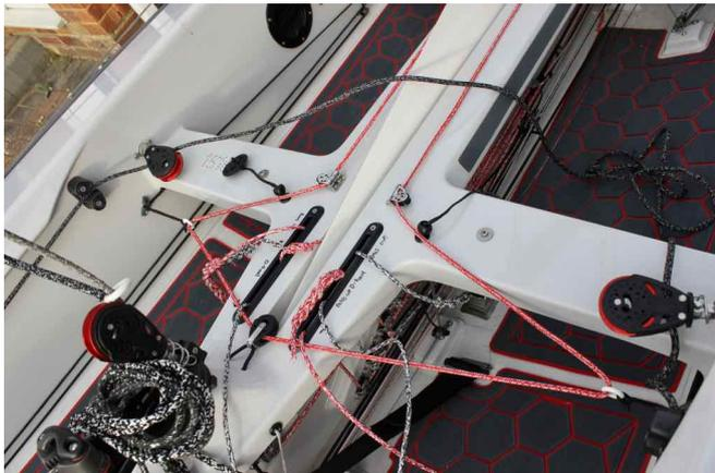
The centreboard control has taken up bringing it to outside of the boat so that again it can be easily found and adjusted by both helm and crew without having to reach inboard or forward.
