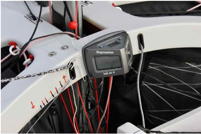
Other controls have been made more accessible starting with the flattener being moved from the boom to the washboard. On the other side of the compass, the pole down has been moved from the centreboard case.
