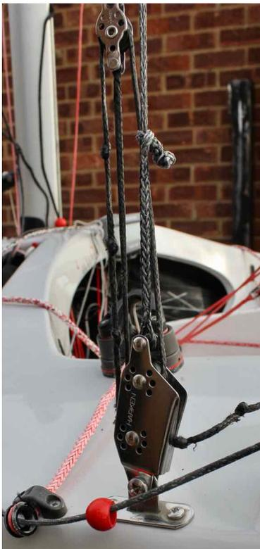
Combined with an adjustable strut, the 'knot system' on the shrouds and a fine tune rig tension led back to the helm has made raking whilst sailing possible. A Ronstan turnbuckle system has made keeping the shroud length equal easy as the knots bed in.
