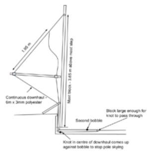
and two bobbles. There is one travelling block running along the bottom of the boat attached to a shock cord retriever. The bobbles come up against the turning blocks by the forward bulkhead to stop the pole skying. (See drawing)
