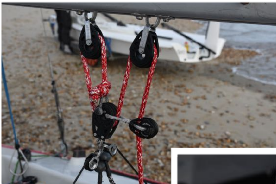
Boom block set up from front of FB (left)
