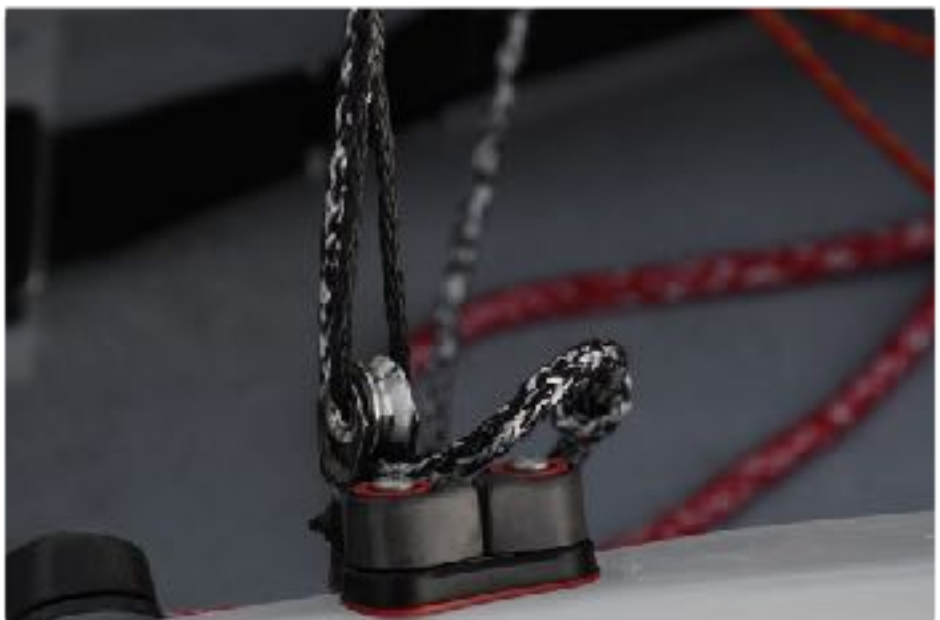
Close up of side tank block (right)
