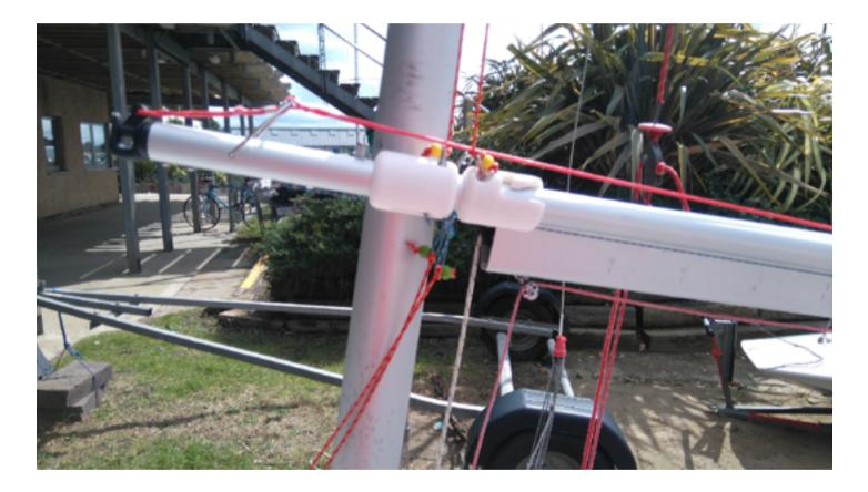
For both the single ended and the Sayce/Rees poles, there are choices with the pole height control. The uphaul(s) can be move so the entry point is higher (~200mm below the jib halyard box?), requiring a sheave fitted here. Alternatively, the uphaul can be fixed to this point and a ring attached to a line entering the mast at the existing sheave point. The uphaul line(s) are passed thru the ring so pulling on the control line puts a kink in the uphaul, effectively shortening it.
